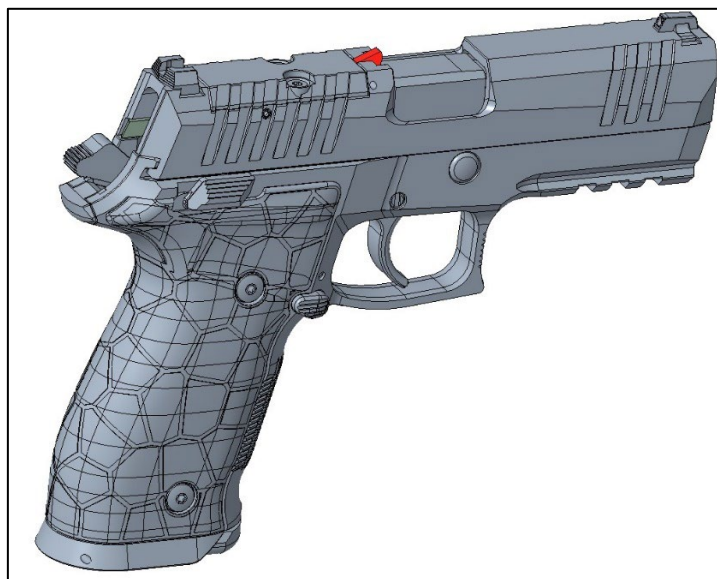
Figure 24: Tactile or visual check of the loaded chamber indicator on slide
