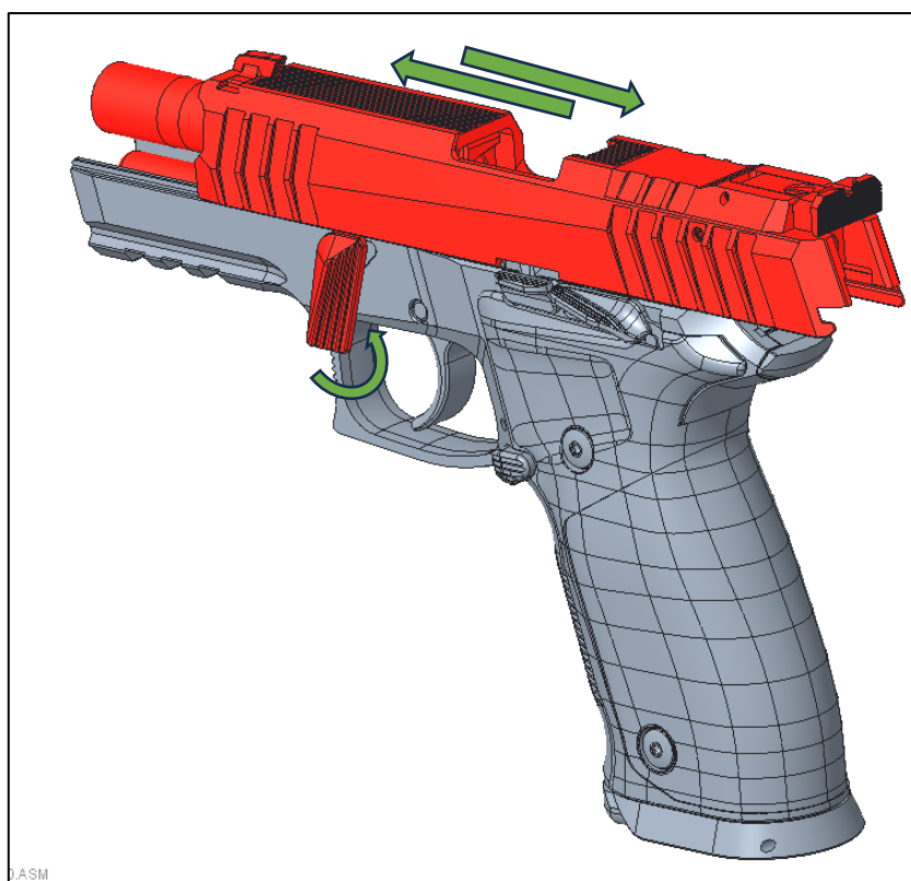
Figure 37: Pulling the slide back until aligned with the frame then turn the disassembly lever to its horizontal position
